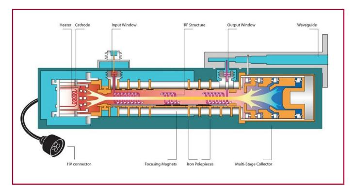
Figure 3. Cross section of traveling wave tube. The cathode and heater at the left.
