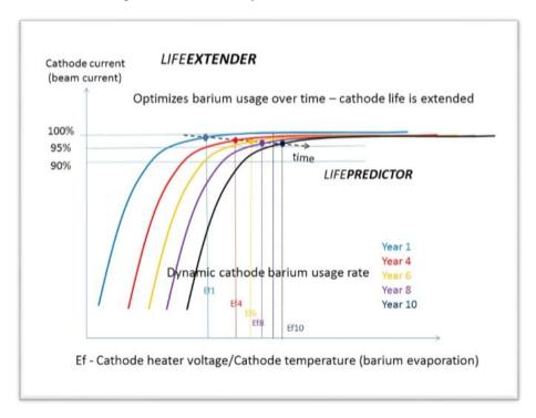
Figure 2. This graph shows the heater voltage increasing over time with LifeExtender, as shown by the six vertical lines, and is set dynamically in order to optimize barium use. This results in 50% longer TWT life.
